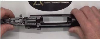
**Step 6**: Now we want to remove the factory trigger sear spring.
