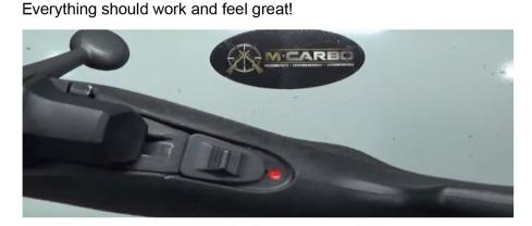
**Step 13**: Try a few trigger pull readings and the M\*Carbo Spring Kit should reduce your trigger pull by half and improve accuracy.
