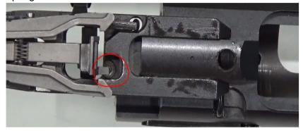
(Replace it with the M\*CARBO Spring Kit using the flathead.)
