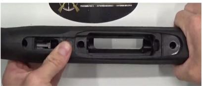
**Step 9**: Screw back on the front screw(shorter) and then place the trigger guard back in. Then tighten back in the screw in the back(longer).
