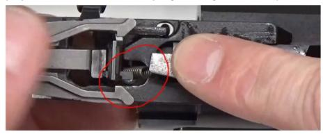
**Step 7**: Pre-travel adjustment. Use the .050 Allen Key to tighten up to your desired amount of travel.
