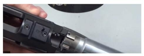
**Step 11**: Do a quick function check then place the weapon on safe then pull the trigger and nothing should happen.
